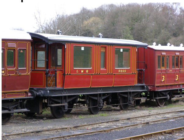
LNWR six-wheel inspection saloon
